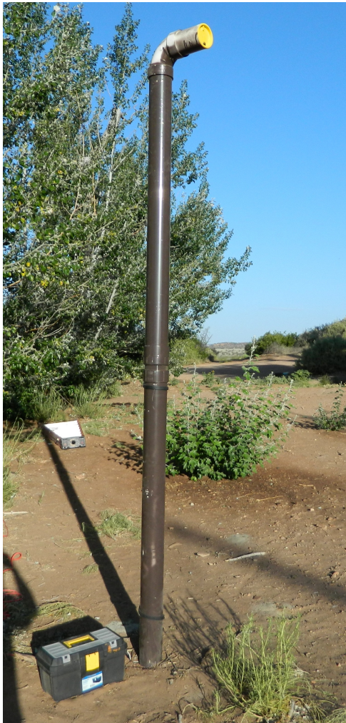
Figure 1. PVC housing for Pettersson D240X. Used in 2012 & 2013 field seasons.
