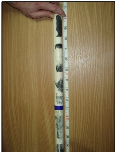
Figure 3. The old MC Spring staff gage next to a measuring tape displaying the equivalent readings on the new staff gage.
