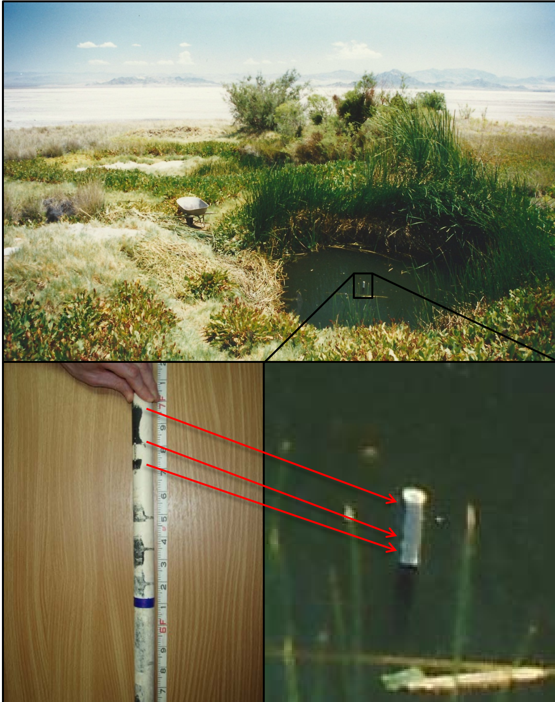
Figure 4. Top: MC Spring in May 1990. Photograph courtesy of Robert Fulton. Bottom: Digitally zoomed-in version of the photograph compared to the old staff gage. The estimated water level for this photograph is 6.65 \pm 0.05 feet.
