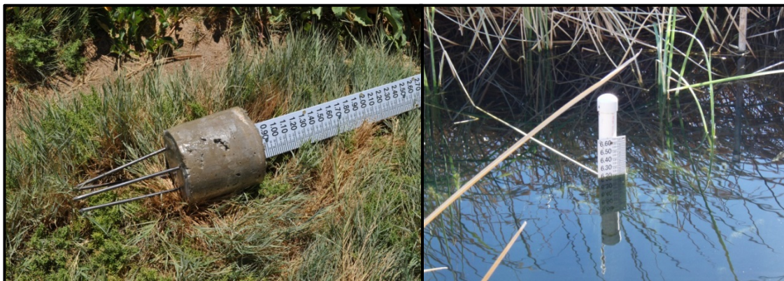
Figure 2. New MOJN I&M staff gage. Left: Staff gage prior to installation. Right: Staff gage on January 15, 2014.
