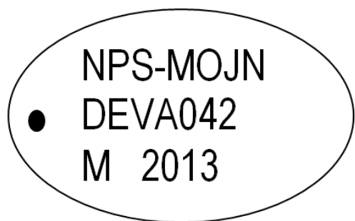
Figure 7.3. Format of metal tags used on the rebar stake marking the corner of the macroplot.
