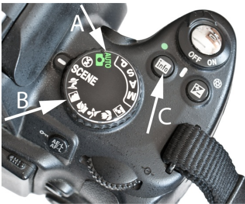
Figure 13.4. Preset settings knob and info button on Nikon D5000 camera. The “auto” (A) and “landscape” (B) settings, and “info” button (C) are indicated by the arrows.
