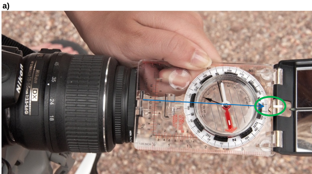
Figure 13.3. Nikon D5000 camera and lens showing how to determine the: a) compass bearing for the camera lens and b) the angle of the camera using the clinometer on the compass. In a), the arrow indicates the direction of the lens to the line of the compass bearing; the number directly under the white line of the compass (circled) is the bearing in degrees. In b), the clinometer reading is circled.
