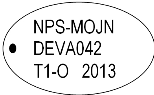
Figure 7.2. Format of metal tags used to mark rebar stakes at the transect ends.
