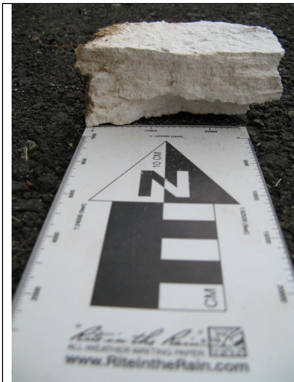
Figure 14. Photograph of top layer exposed in a trench. This layered sediment easily breaks by hand.
