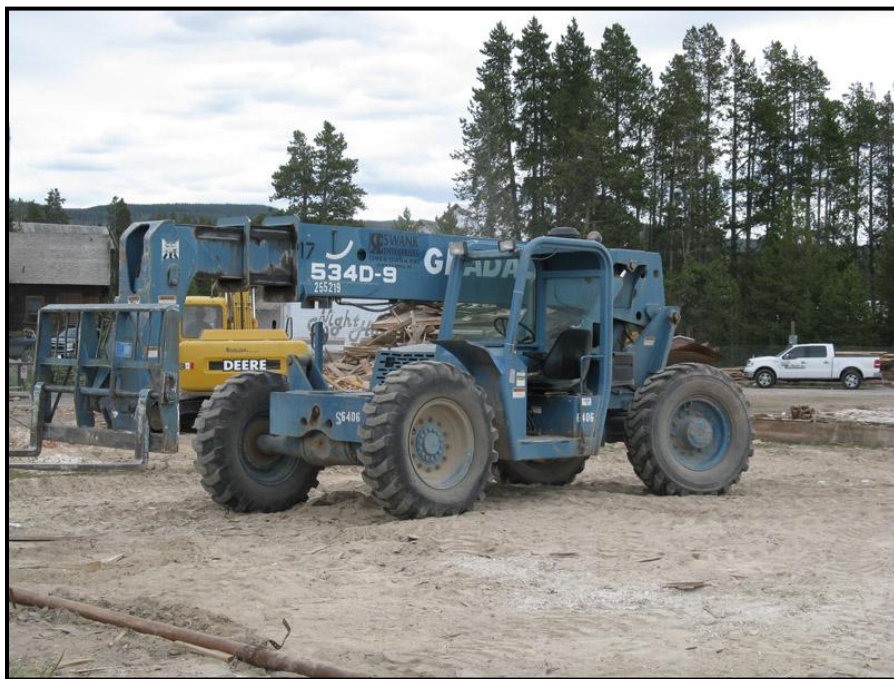
Figure 13. Photograph of fork lift that twice broke the ground surface into active thermal ground on 12 August 2009 between 3 to 3:30 p.m. MDT. Photograph taken 18 August 2009. Location of the two breakthroughs are shown in Figure 8 noted by the 152 °F (67 °C) temperatures outside the northeastern edge of the building.
