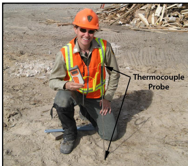
Figure 11. The Oakton Acorn thermocouple-thermometer using a type K thermocouple probe that is a hollow ¼ inch (6.4 mm) diameter, stainless-steel tube, 41 inches (104 cm) in length. Photograph was taken in the construction area on 18 August 2009. Chelsea Feeney, Geological Society of America Geocorps volunteer, is measuring temperatures at 10 inches (25 cm) depth.
