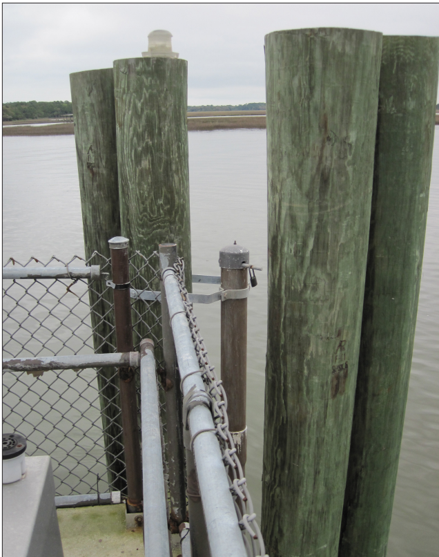
Figure 4. Continuous data collection platform used at Timucuan Ecological and Historic Preserve (TIMUking). Photo shows sonde housing and locking cap. Photo by Peter Mockus, SECN Staff.
