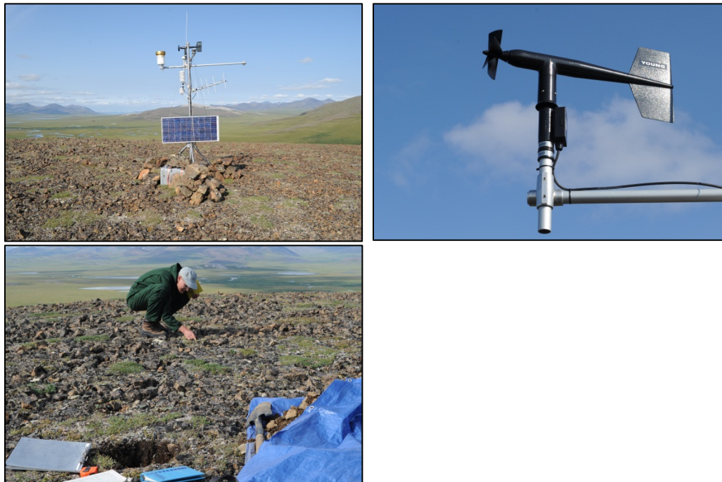
Figure 6. Howard Pass, July 25, 2015 (top left). New alpine WS-WD sensor (top right). Soil pit and vegetation classification (bottom).
