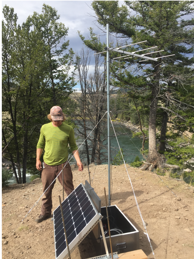
Figure 2. Fixed radio telemetry station located at the confluence of the Lamar and Yellowstone River, September 2015.
