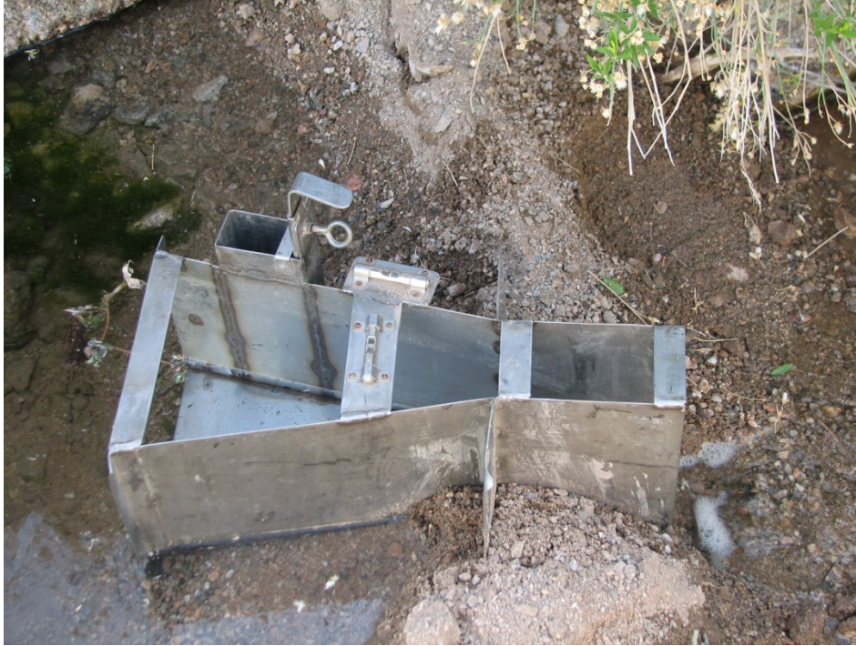
Figure 7.1. Portable flume deployed at Burro Spring in LAKE. Photo by G. Karst.
