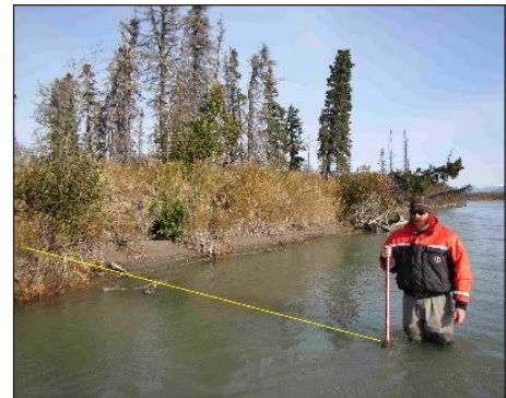
Figure 23. Jeff Nelson balances a sledgehammer on rebar anchoring a newly deployed HOBOT in the Savonoski River on October 1, 2014. The yellow line indicates the distance from the base of the vertical part of the bank to the rebar.
