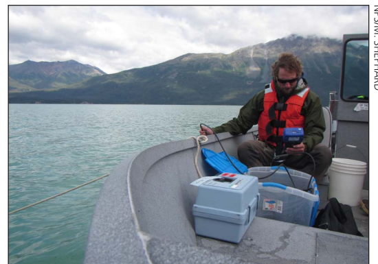
Figure 6. Evan Booher samples core parameters with the EXO2 multiparameter sonde in Lake Clark on July 15, 2014.
