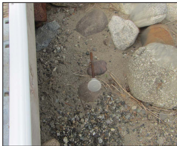
Figure 11. The NOAA-NWS marker used for tape-down measurements of stage at the Naknek Lake outlet. Measurements were made from the base of the rebar. Photo taken June, 2014.
