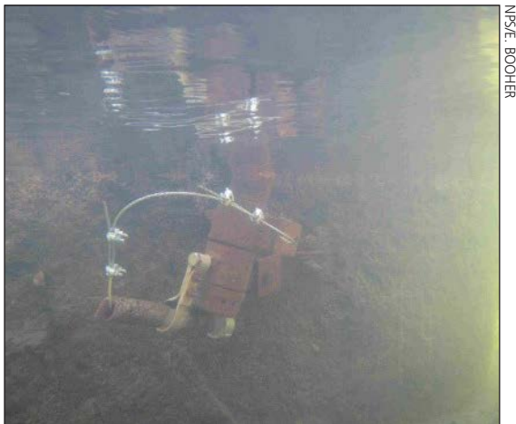
Figure 12. Installation of the In-Situ level logger on the remains of the USGS staff at the Naknek Lake outlet on May 23, 2014. The staff was damaged by ice during the 2013-2014 winter.
