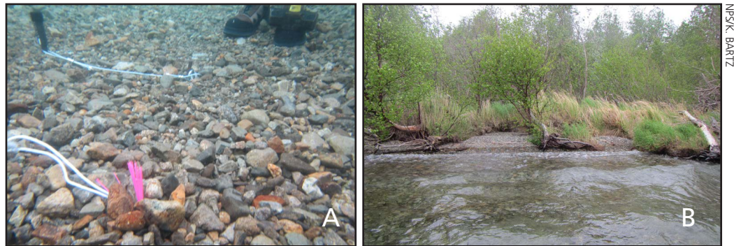
Figure 27. Underwater view of the interstitial (foreground) and surface (background) temperature logging devices installed in Kijik Lake on May 29, 2014 (A). View of the lake shore from the logger location, showing the live (left) and dead (right) birch trunks (B).
