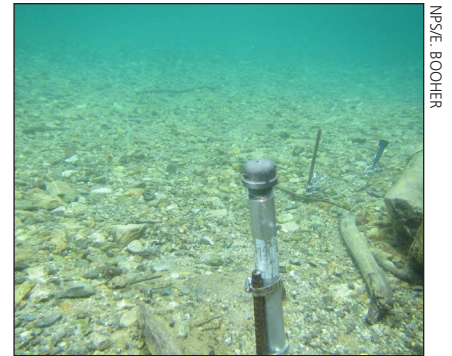
Figure 16. Housing for the In-Situ level logger, attached to rebar and installed in the Little Kijik River on May 28, 2014. The Onset HOBO Water Temp Pro v2 (intended for continuous, year-round water temperature monitoring) is visible in the background.
