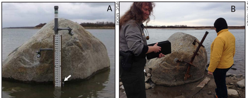
Figure 10. Past (A) and present (B) photos of the staff gage and level logger (white arrow in A) on “To Go Rock,” located upstream of the boat dock at Lake Camp on the Naknek River.
