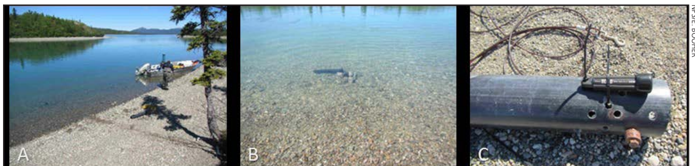
Figure 3. Installation site of the multiparameter sonde for continuous water quality monitoring at the Lake Clark outlet on June 3, 2014 (A). The sonde was cased in in PVC housing and anchored to the substrate (B). Attached to the PVC housing was a HOBO data logger, to initiate continuous year-round water temperature monitoring at the Lake Clark outlet (C).
