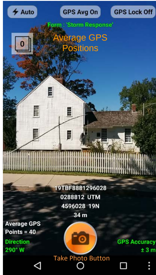
Figure 2. Screen depicting the GeoJot APP being used to collect a photo with coordinates and attributes. Note that the photo coordinates can be averaged to improve the photo coordinate. In this case, 40 GPS fixes were averaged to calculate a coordinate with an accuracy of \pm 3 m.
