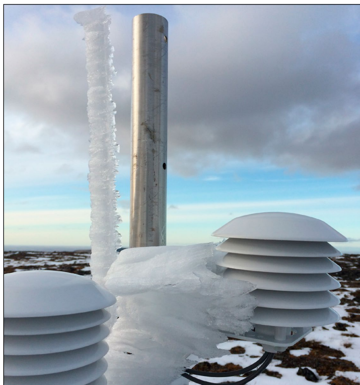
Figure 8. Rime ice at the downsized Midnight Mtn station in September 2014. During the formation of the ice, wind was blowing from left to right.
