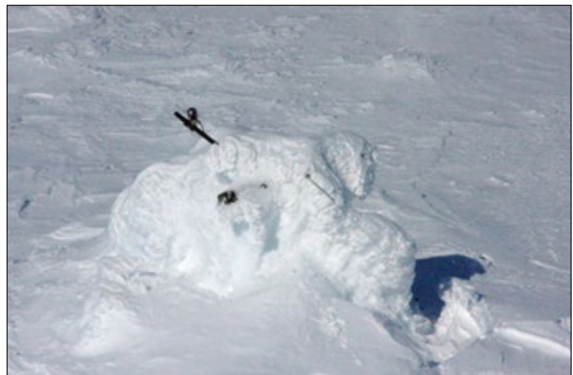
Figure 6. An extreme rime ice example at the Midnight Mountain meteorological station in 2012. The ice encased and destroyed the 10-foot tall tripod. The station was downsized in 2013 and now only measures air and soil temperatures. (photo Walker Gusse)
