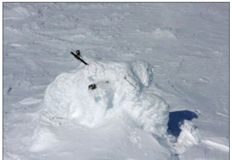
Figure 6. An extreme rime ice example at a meteorological station on the Seward Peninsula in 2012. The ice encased and destroyed the 10-foot tall tripod. (photo Walker Gusse)
