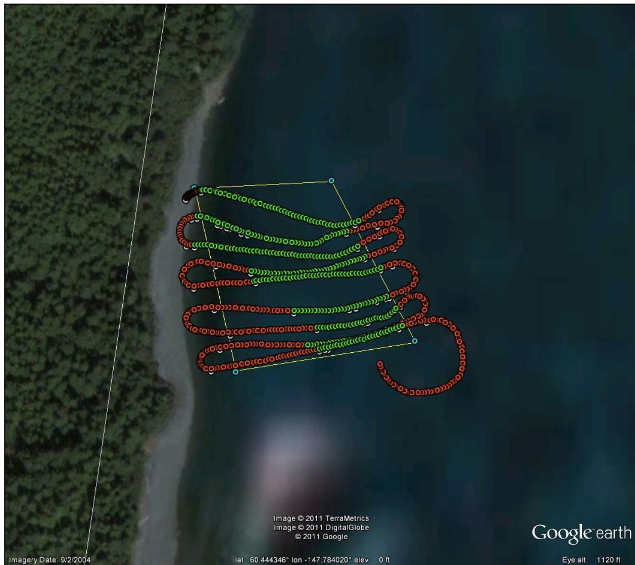
Figure 4. Example plot of sonar transects. The yellow line indicates the boundary of the prescribed sampling area at this site; red dots indicate sonar soundings where no eelgrass was observed; and green dots indicated sonar soundings where eelgrass was found.
