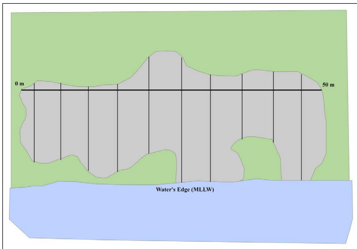
Figure 2. A hypothetical mussel bed including one horizontal 50 m baseline transect (bold) and 10 variable length vertical transect lines that extend from the upper margin, to the lower margin of the bed (or zero tidal elevation if bed continues below MLLW). The vertical transects are 5 m apart from the first randomly located vertical transect and are variable in length, depending on the width of the mussel bed.
