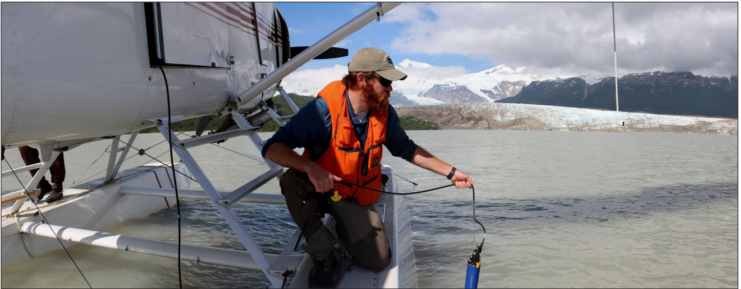
Hydrological technician, Jeff Nelson, samples water quality with a multi-parameter sonde in Hallo Glacier Lake, Katmai NPP.
