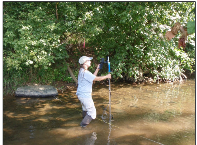
NCRN Hydrologic Technician Tonya Watts takes flow measurements during water quality monitoring at Monocacy National Battlefield. NPS Photo.
