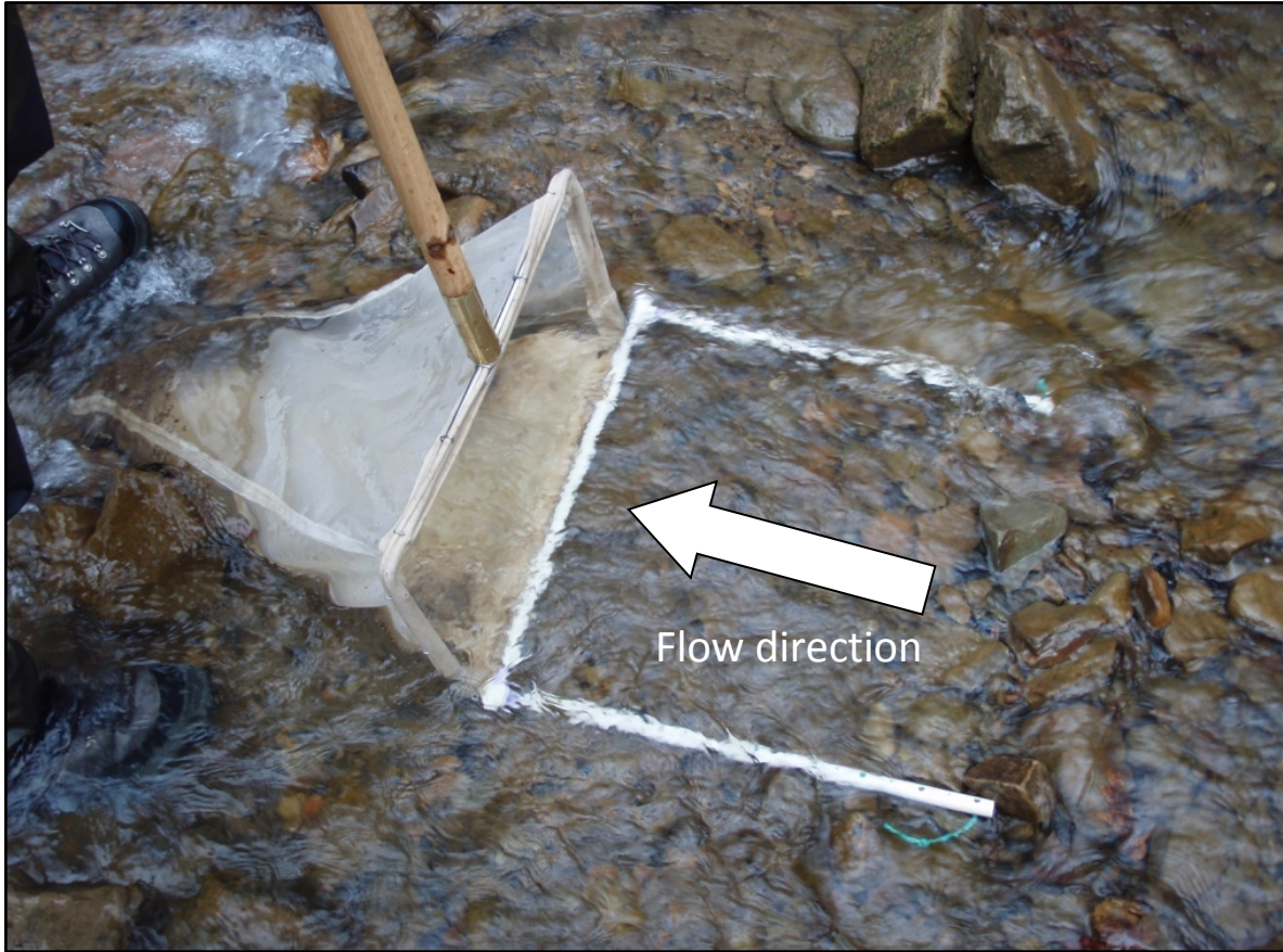
Figure 1. Correct positioning of the Slack Sampler and 0.25 m 2 area template relative to stream flow direction.
