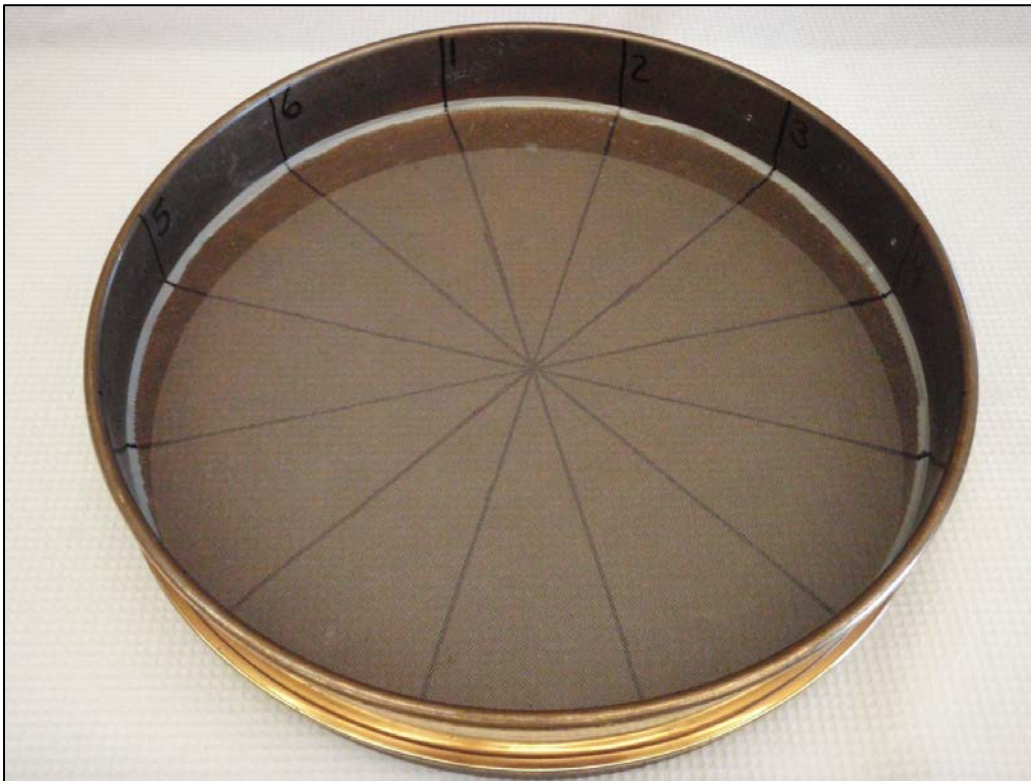
Figure 3. Metal sieve (30 cm diameter; 500-µm screen) used for benthic macroinvertebrate sample splitting. The sieve is marked with six equally spaced (30 degrees apart) diameter markings that are extended up the inside walls of the sieve and numbered 1 through 6.
