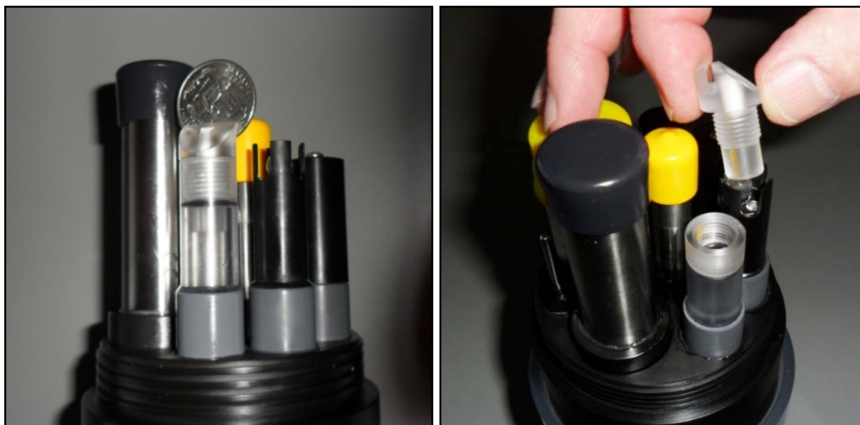
Figure 2. To remove the pH reference electrode cap, insert a coin or appropriate screwdriver into the slot on the cap to loosen it (left) then unscrew and remove it using your fingers (right).
