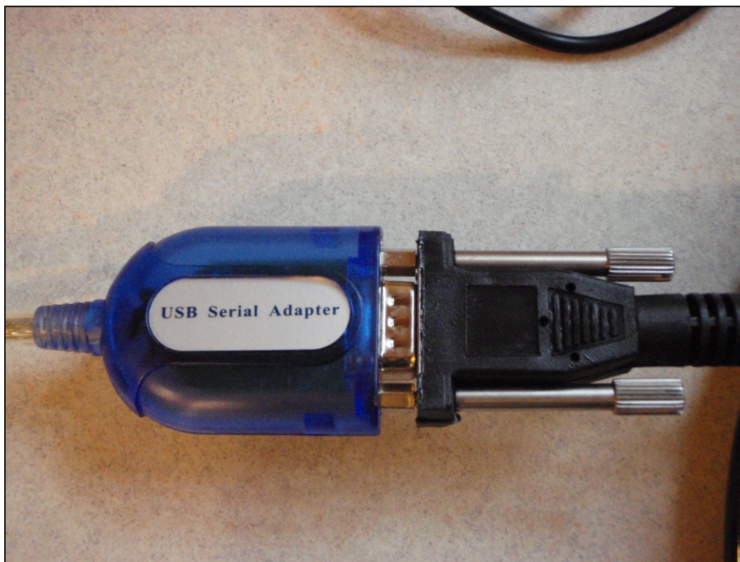
Figure 1. Adapter used for connecting Eureka multiprobes to USB port on personal computers.
