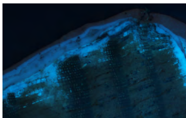
Figure 22: Sample ELK.7.1, 40x magnification, visible light (above) and UV light (below). The wood surface is worn and discolored, and the early green paint is soaked into the wood.
