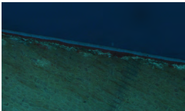
Figure 28: Sample ELK.8.5, 40x magnification, visible light (above) and UV light (below). The brown layer (arrow) is autofluorescent and may represent a resinous finish.
