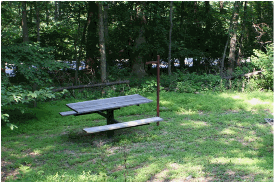
The new type of picnic tables are mounted on a single tubular metal post set within a concrete footing. (2012 Peaks of Otter Cultural Landscape Report)
