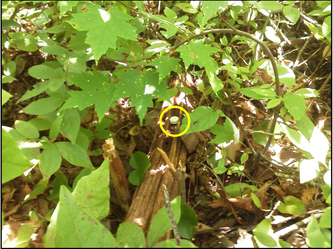
Figure 2.10: Surface temp measurement - understory cover. Due to steep topography and curious wildlife, sensors (circled) were placed on a flat portion of woody debris stabilized by split twigs staked out around the periphery.
