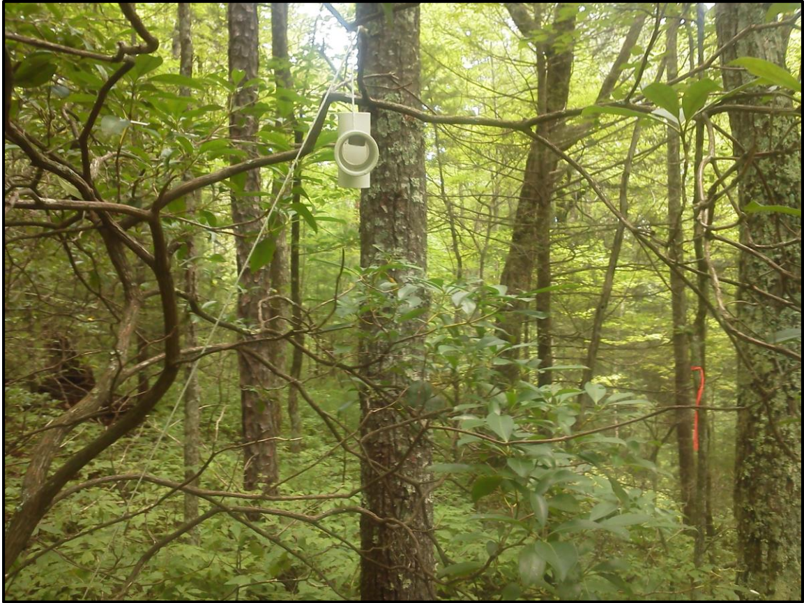
Figure 2.11: Air temp and humidity measurement. The Ibutton (grey cylinder underhanging top of open PVC) is hung at 2m and receives ample atmospheric contact. The vertical PVC tube (white string attached) allows precipitation to pass through the housing without direct contact with the sensor. The white color reflects solar radiation, providing accurate readings of air temperature and humidity.
