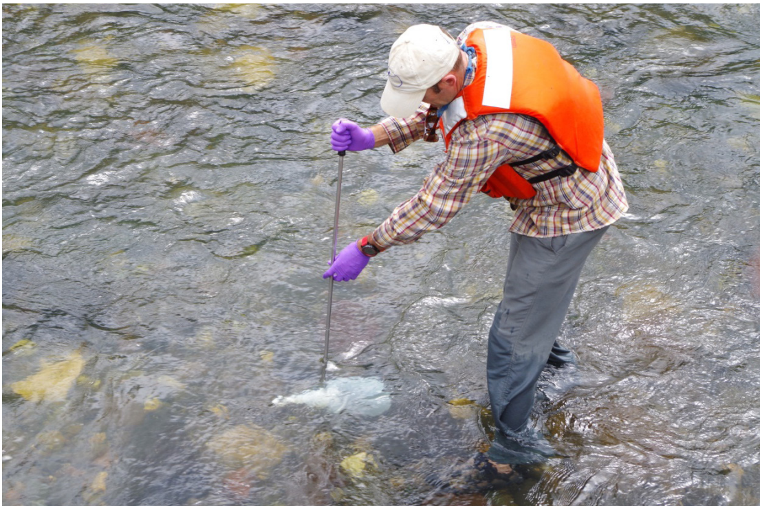
Photo 3. River sampling is accomplished with a DH-81 Sampler affixed to a 1-m wading rod with 3-L bottle during wadeable conditions. Photo from the Lamar River near Tower Ranger Station, WY.
