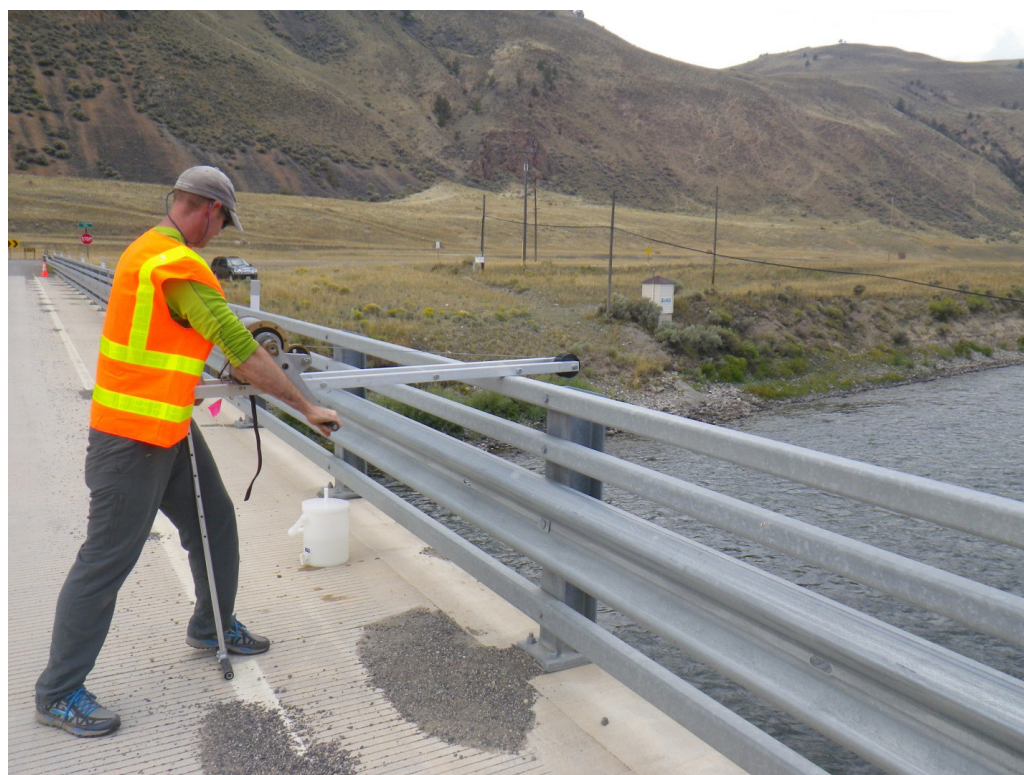
Photo 1. River sampling is accomplished using a bridge board, reel, and churn splitter during high flows and within large rivers (e.g., Yellowstone River at Corwin Springs, MT).
