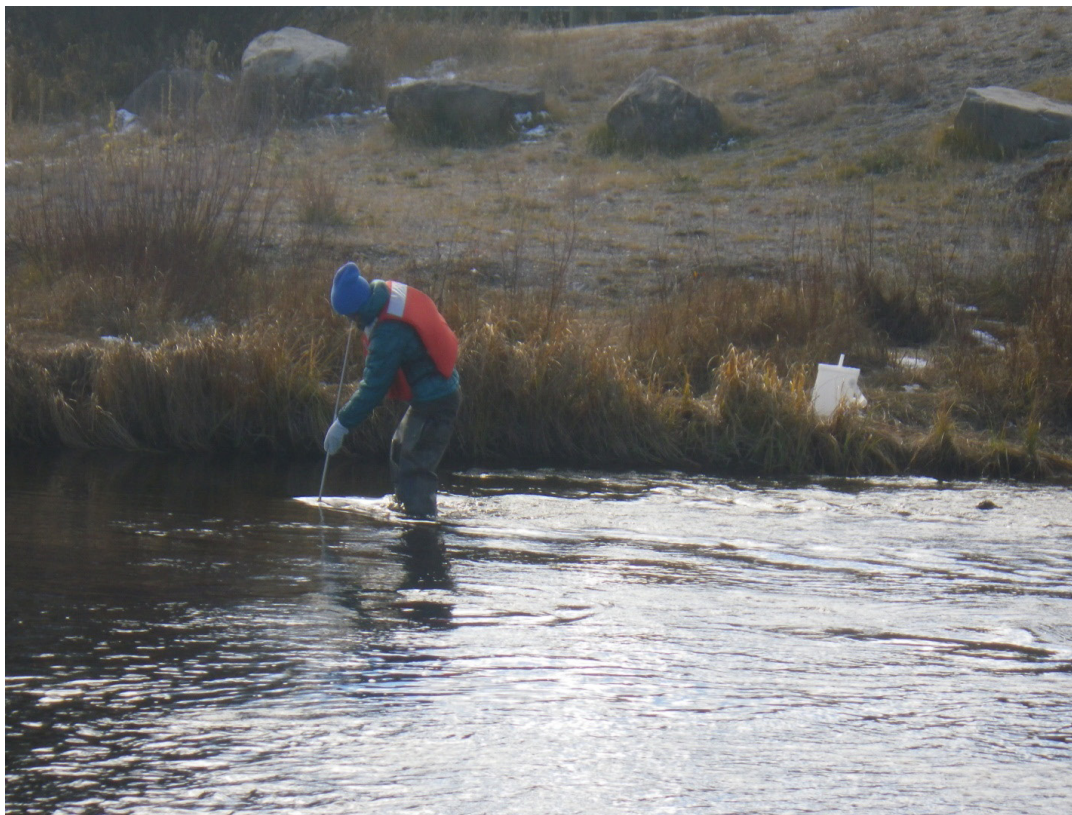
Photo 2. River sampling at the Madison River sampling location. Width- and depth-integrated techniques are used and collected water is composited with an 8-L polyethylene churn splitter to produce a representative sample of river conditions.
