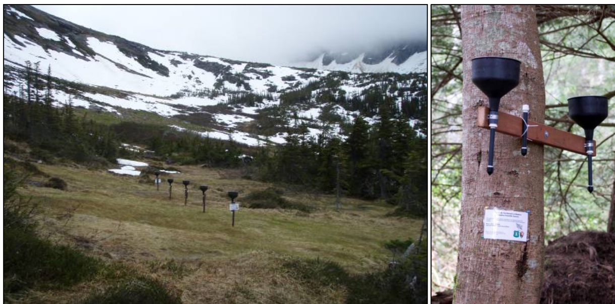
Figure 2. Open (OD; left) and throughfall (TD; right) ionic exchange resin tube (IER) deposition samplers deployed in KLGO during the summer of 2008 (Schirokauer et al. 2014).
