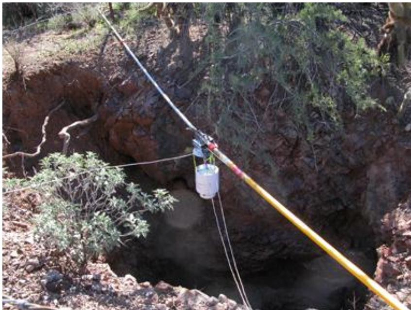
Remotely-controlled downhole camera used to inspect shafts for the presence of drifts.
