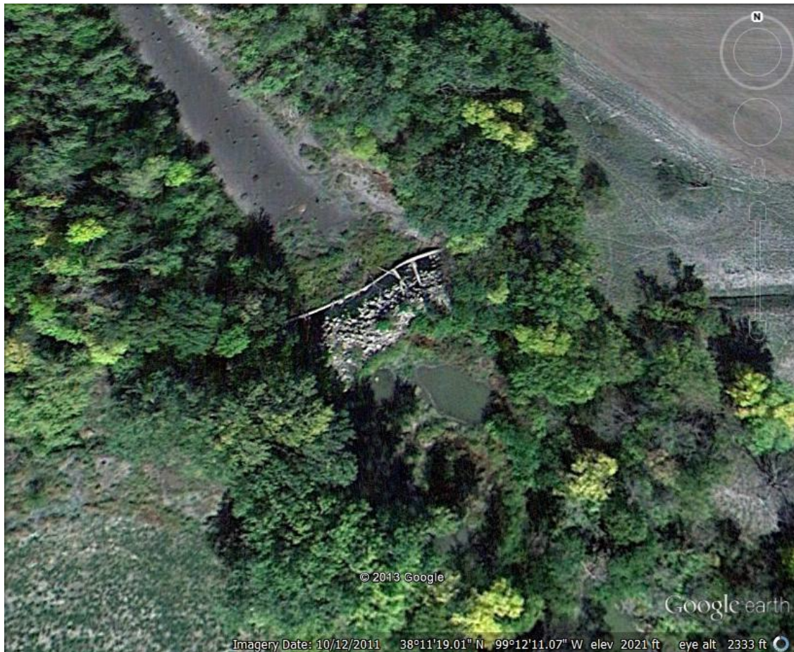
Figure 5. Oblique aerial Google Earth image of the check dam that spans the channel of the Pawnee River about 500 feet downstream of the park boundary. Note the pool of open water downstream of the dam, which suggests a connection to the local water table at that elevation.
