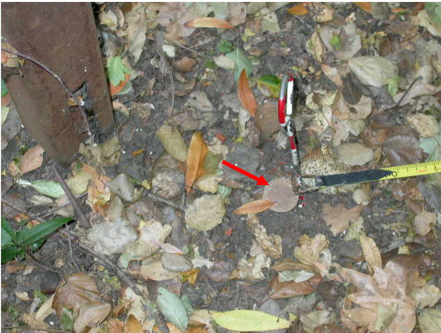
Photo 5: Close up of right-bank monument XS2 (brass cap) with temporary red-and-white chain pin
