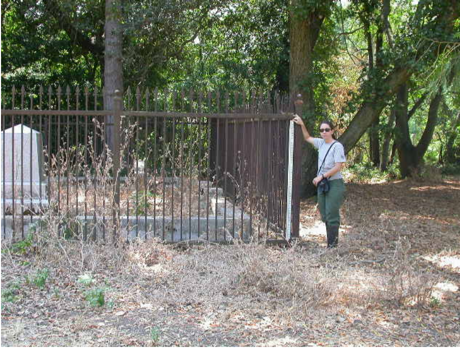
Photo 10: Location of reference point for measurement of creek bed elevation (rod sits on top of the bottom rail of the fence)
