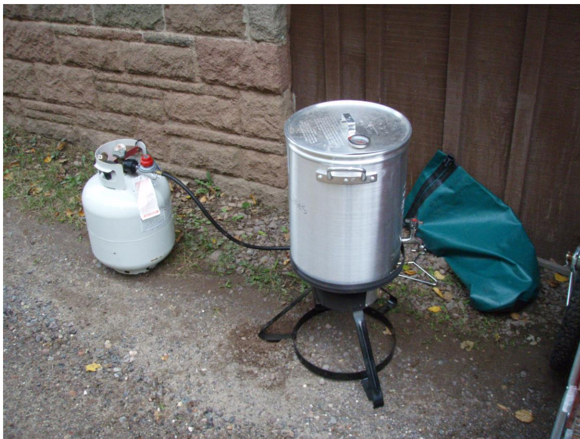
Figure 5-1. An example of a propane burner and pot used to heat water to 140° F (60° C) for decontaminating non-electronic equipment. Any large pot and heat source is acceptable; however a thermometer should be used to verify that sufficient temperatures have been achieved.
