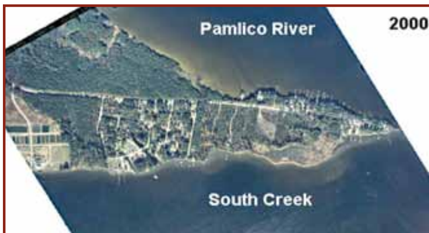
FIGURE 8-4-6. The Hickory Point and Pamlico Marine Lab site aerial photograph time slices for 1970, 1984 and 2000. The marsh shoreline on the South Creek side of Hickory Point has two small clumps of upland trees (dark zones) forming small headlands on the south side of the marsh in the 1970 aerial photograph. In the 2000 photograph, these two areas of upland vegetation are completely eroded away, and the shoreline is beginning to straighten out in response to the erosion processes. Notice the increased rate of shoreline hardening from 1970 to 1984, in concert with a significant recession of the unmodified low sediment bank shoreline west of Hickory Point along the Pamlico River shore (see Fig. 8-4-5).
