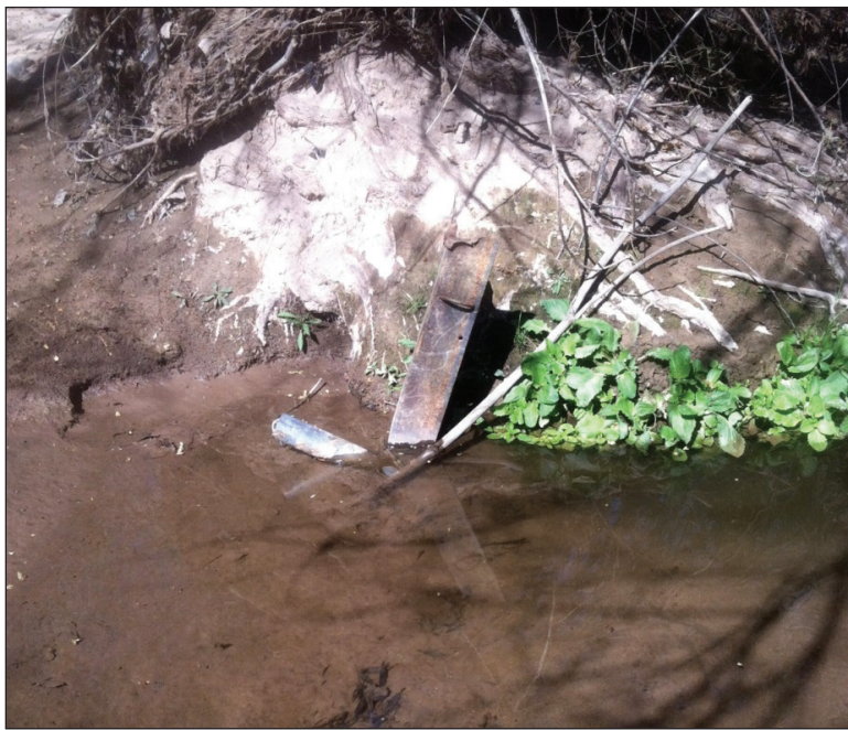
Figure 4-7. Sonde mount (a ~2-m steel beam driven into the sediment of the river bottom) at the Santa Gertrudis index site at Tumacácori National Historical Park. This mount was previously in the active channel, with the stream bottom approximately 0.75 meters below the elevation depicted in the photograph.
