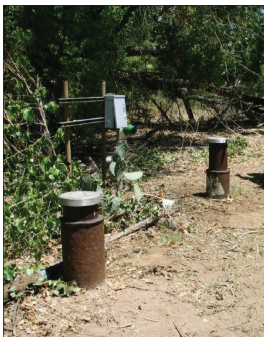
Figure 3-3. Monitoring wells prior to installation (left; MW-1 Deep in the foreground, with MW-1 Shallow) and following instrumentation of real-time measurements (right; white box encloses MW-1 Deep), Tumacácori National Historical Park.
