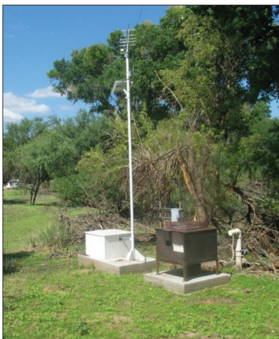
Figure 3-3. Monitoring wells prior to installation (left; MW-1 Deep in the foreground, with MW-1 Shallow) and following instrumentation of real-time measurements (right; white box encloses MW-1 Deep), Tumacácori National Historical Park.
