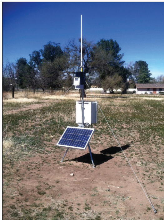
Figure 2-1. The Davis real-time weather station at Tumacácori National Historical Park. Data are available through www.climateanalyzer.org .
