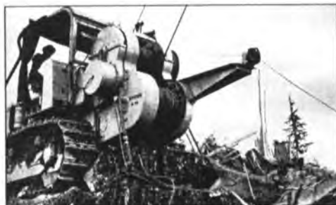
B1. A Caterpillar D-9 equipped with Hyster D98A Yarder attachment
