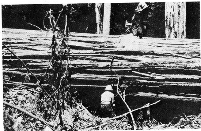
Bucking required a team of men. The man on top of the tree used a 7' bar which is visible, while the man on the ground is completing the cut with a 5' bar.
