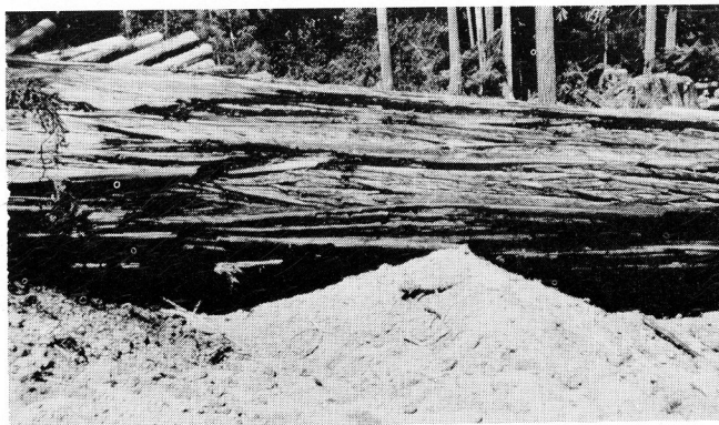
This is the cable in position ready for the final cut, with the tree in tension. A drum line, \frac{7}{8} -inch, and 240' long is used in conjunction with 125 feet of tree rigging line.
