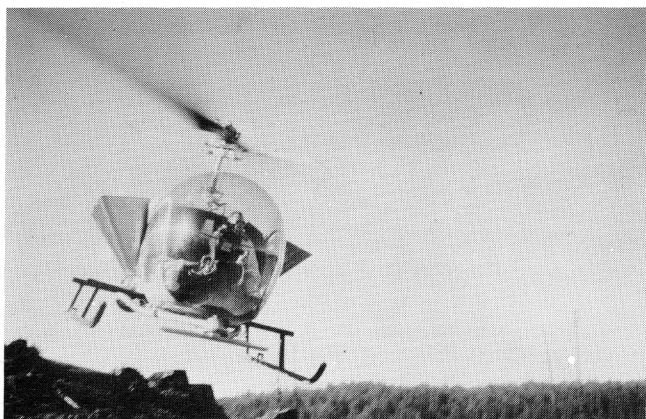
Helicopter at center near the reference tree. Flight is at an elevation of 200 feet, swath width is 120 feet, coverage is 8 acres per minute.
