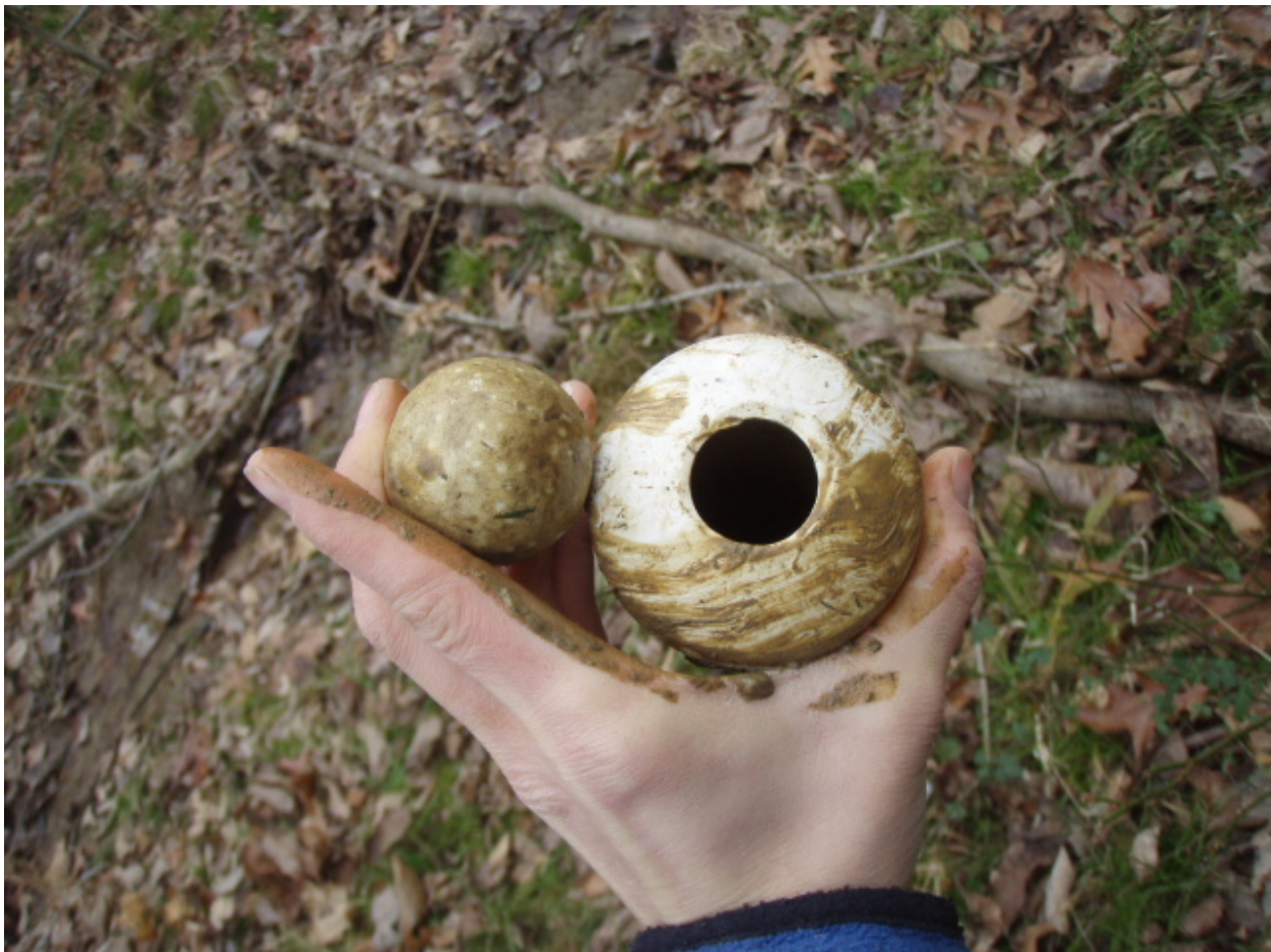
Figure 7.2. The three essential components of our handmade well bailer include a 3" PVC pipe, a well cap with a hole, and a golf ball.
