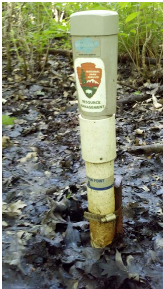
Figure 7.4. Wells can be clamped to angle iron that is driven into consolidated ground, to prevent movement. All 40-inch Ecotone water level loggers are reinforced with angle iron. The dark blue line is the calibration point.
