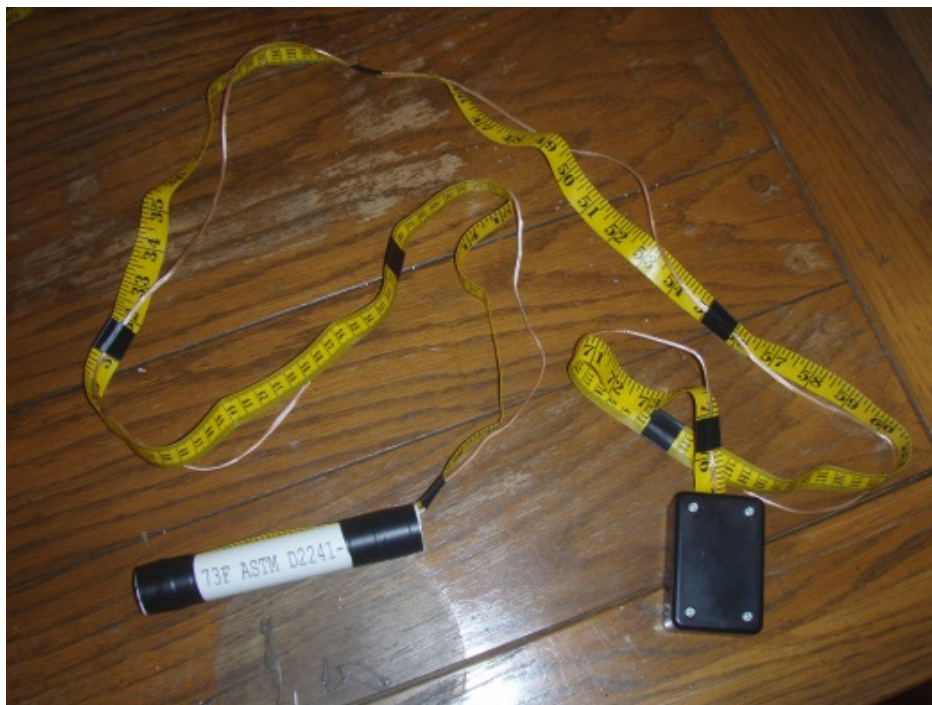
Figure 7.5. The basic construction of a hydrolite or hydrobuzzer used to measure water table depth in manually-measured groundwater wells.
