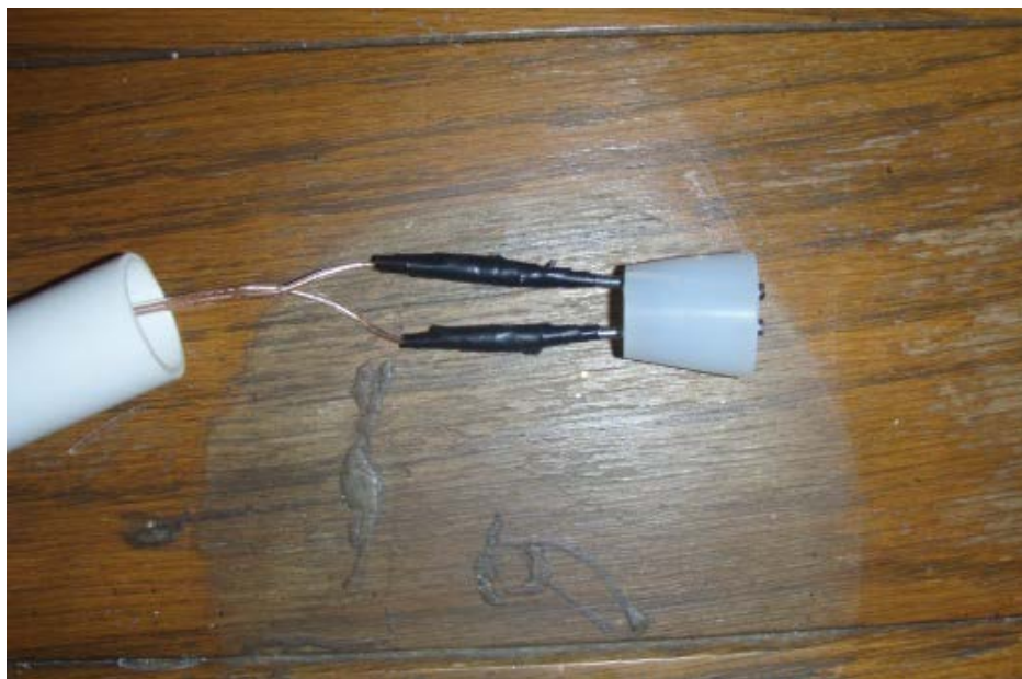
Figure 7.6. Speaker cord is attached to the nail "sensors" with electrical tape and protected inside a piece of PVC with rubber stoppers.
