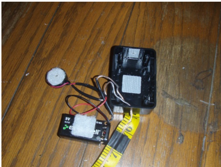
Figure 7.7. The LED light (or buzzer) is connected to the 9V snap connector and one section of the stripped speaker cord. The other section of stripped speaker cord attaches to the other 9V snap connector.
