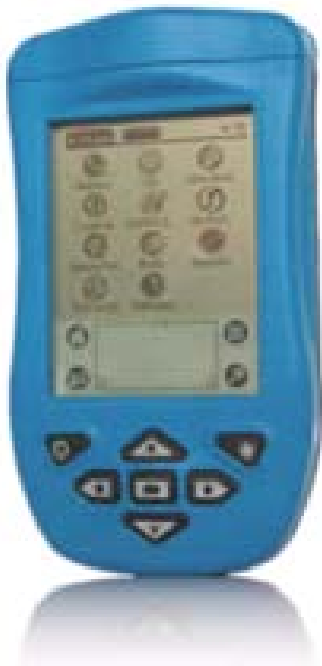
Figure 8.4. The Aceeca Measura Rugged Digital Assistant (Measura) is used to download data from Ecotone water level loggers and then to upload the data to a desktop computer.
