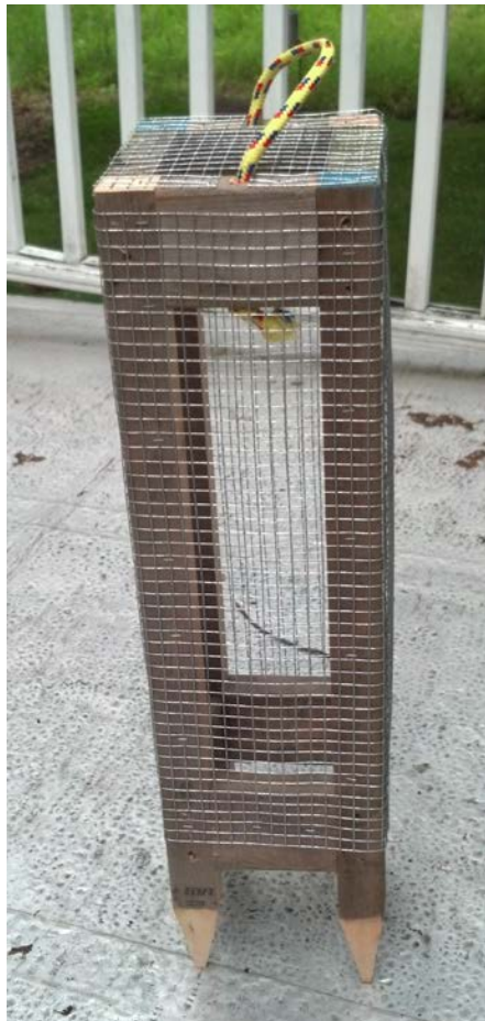
Figure 8.3. The beaver deflector used to protect Ecotone water level loggers from animal vandalism.
