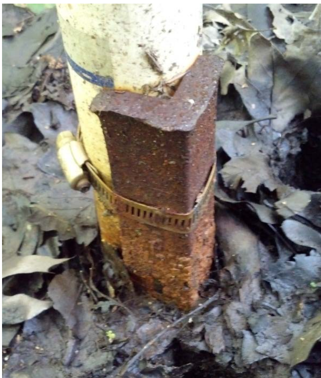
Figure 8.1. All 40-inch Ecotone water level loggers are reinforced with a 10-inch piece of angle iron and secured with a hose clamp.
