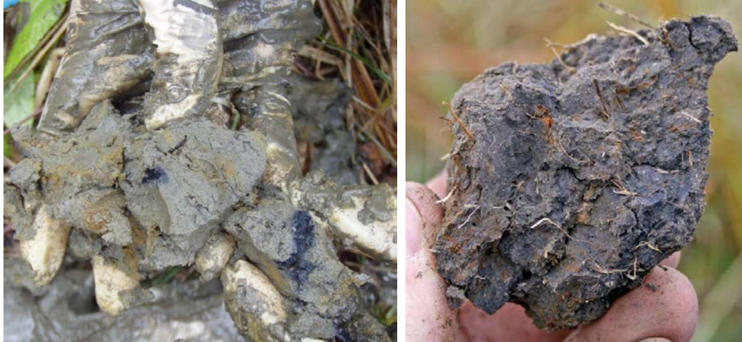
Figure 10.2. a) An example of a sandy, reduced soil with a gray (gleyed) matrix with orange and black streaking (mottles). b) A mineral soil with a gleyed matrix and oxidized roots (USACE Midwest Regional Supplement 2010).
