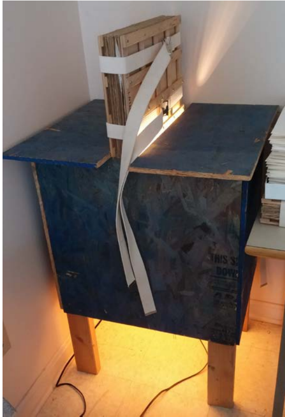
Figure 13.1. The plant press dryer is used to quickly dry out plant specimens held in a wooden press.
