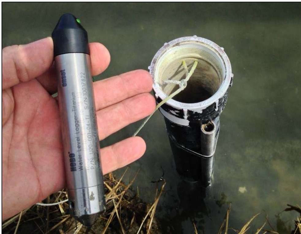
Figure C 5. Water level sensor and PVC housing (Fire Island National Seashore).
