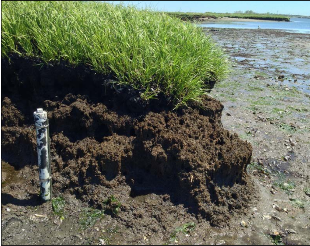
Figure C 4. Water level housing next to a wetland (Jamaica Bay, Gateway National Recreation Area).
