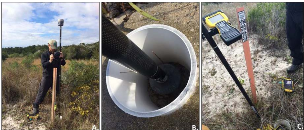
Figure 32. A. Taking a measurement at a Check-In. B. A close up of the rover pole on the bench mark. C. Locating local bench marks for Check-Ins ensures the accuracy of surveys.
