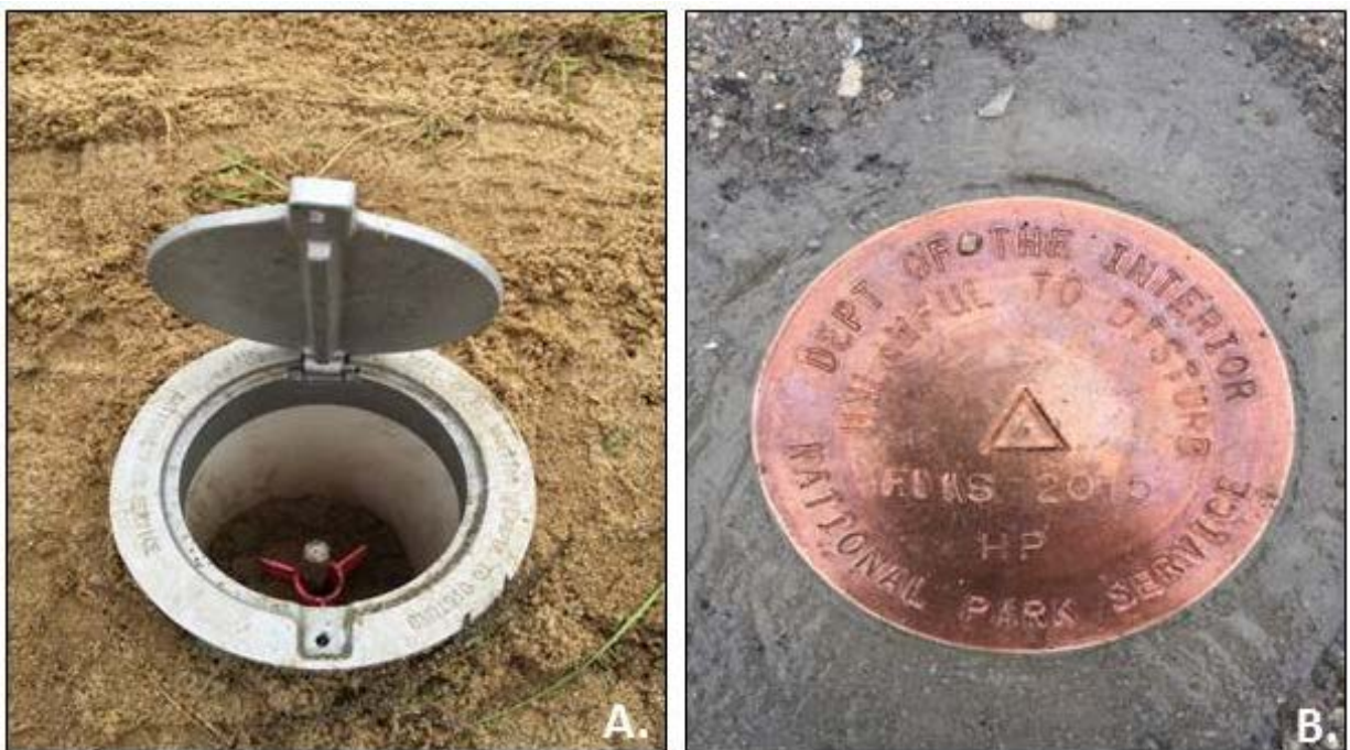
Figure 20. A. bench mark in the form of a steel rod driven to refusal. B. A bench mark in the form of a brass disk encased in concrete in a solid structure.
