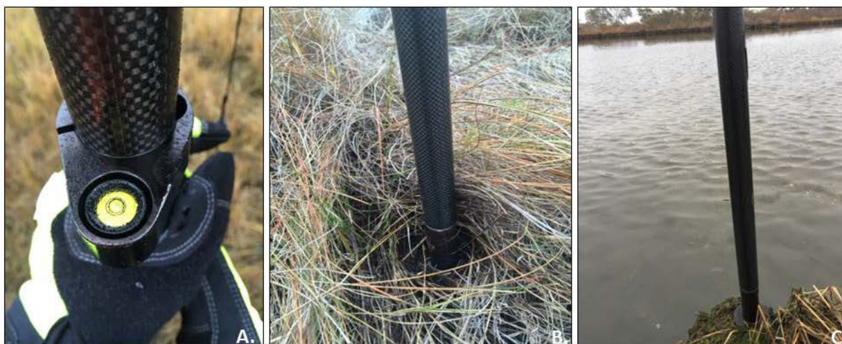
Figure 31. A. Keep the rover pole as level as possible. B. Make sure the rover pole is resting on the marsh surface (bare earth). Move thick vegetation, algal mats, or wrack out of the way. C. If a grid point falls within a creek, ditch, or bay; measure the point on the edge of the marsh surface closest to the grid point.
