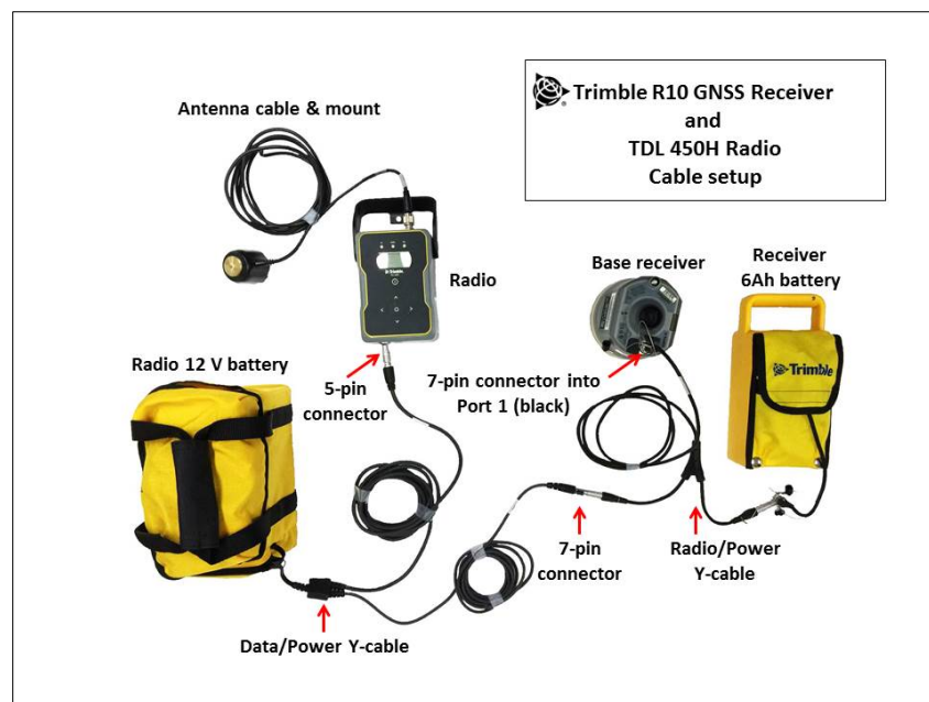
Figure 25. Simplified schematic of cables and devices connecting a base receiver with an external radio.
