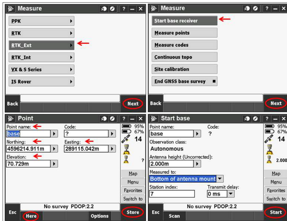
Figure 24. Starting a base receiver in Trimble Access. The antenna height should be carefully recorded and double checked to ensure correctness.
