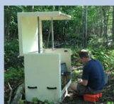
Figure 3: Flow monitoring instrumentation was installed at the bottom end of Cromwell Brook containing water depth sensors, velocity sensors and a pump sampler for the measurement of total suspended solids concentrations.
