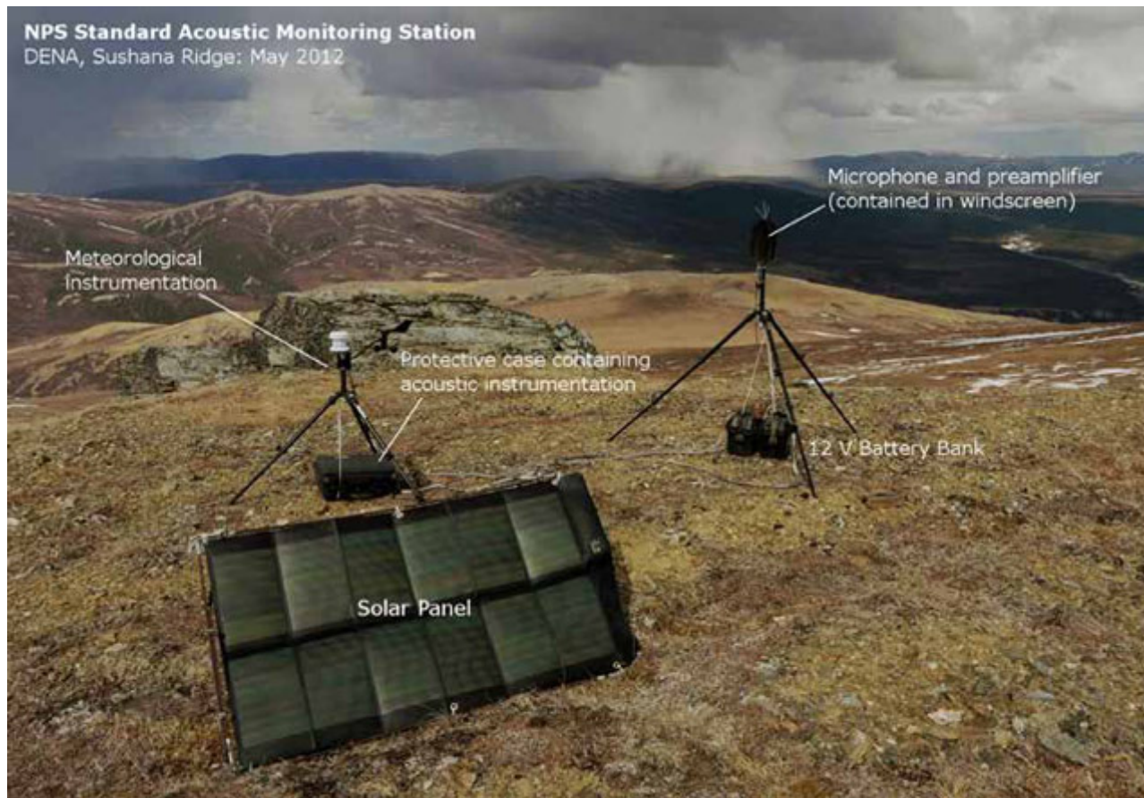
Figure 2. Photograph of a standardized NPS acoustic monitoring station, deployed in Denali National Park atop Sushana Ridge, May 2012.
