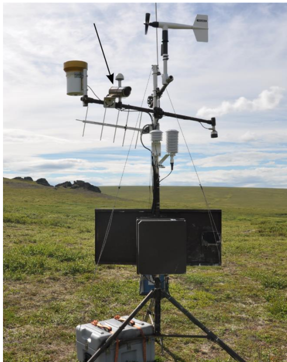
Figure 6. Typical phenology camera setup. The camera is the metal cylinder marked with an arrow. Climate monitoring instruments are also attached to the tripod. The solar panel is visible facing away from the photo lower on the tripod. This is the Serpentine Hot Springs climate station in BELA.
