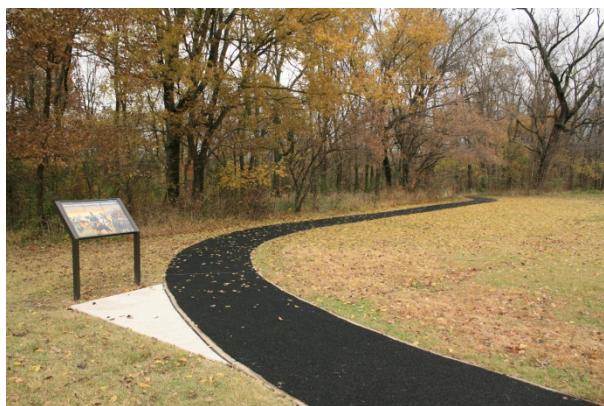
FIGURE 101. A portion of the trail features a rubberized surface set over concrete.
