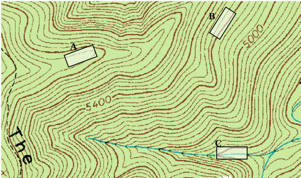
Figure 1. Proper orientation of plots on the landscape. The centerline should run parallel to ridges (A), parallel to contours (B), and parallel to streams (C).
