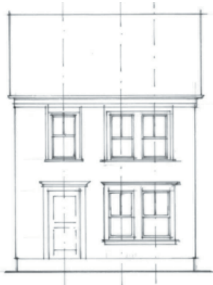
Windows usually stack to maintain the structural integrity of the load-bearing walls, which transfer structural loads down between the openings.
