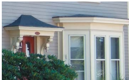
Metal roofing is common on low pitches over porticos, porches and bays.
