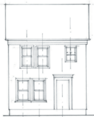
Windows usually stack to maintain the structural integrity of the load-bearing walls, which transfer structural loads down between the openings.
