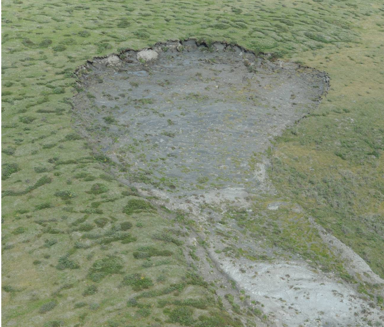
Figure 6. A retrogressive thaw slump in the Noatak National Preserve. The escarpment at the upper end of this slump is advancing into undisturbed tundra as the ground thaws, material falls onto the slump floor, and slides downhill.
