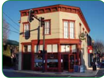
EXAMPLE OF INAPPROPRIATE TREATMENT: REMOVAL OF HISTORIC STOREFRONT CORNICE
