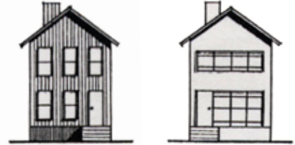
INAPPROPRIATE FAÇADE FENESTRATION AND ARTICULATION
