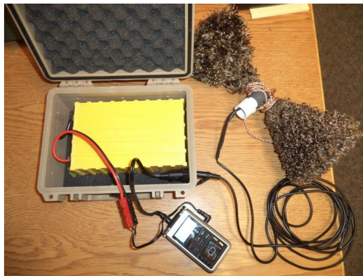
Figure 2. Components of a biological sound station
