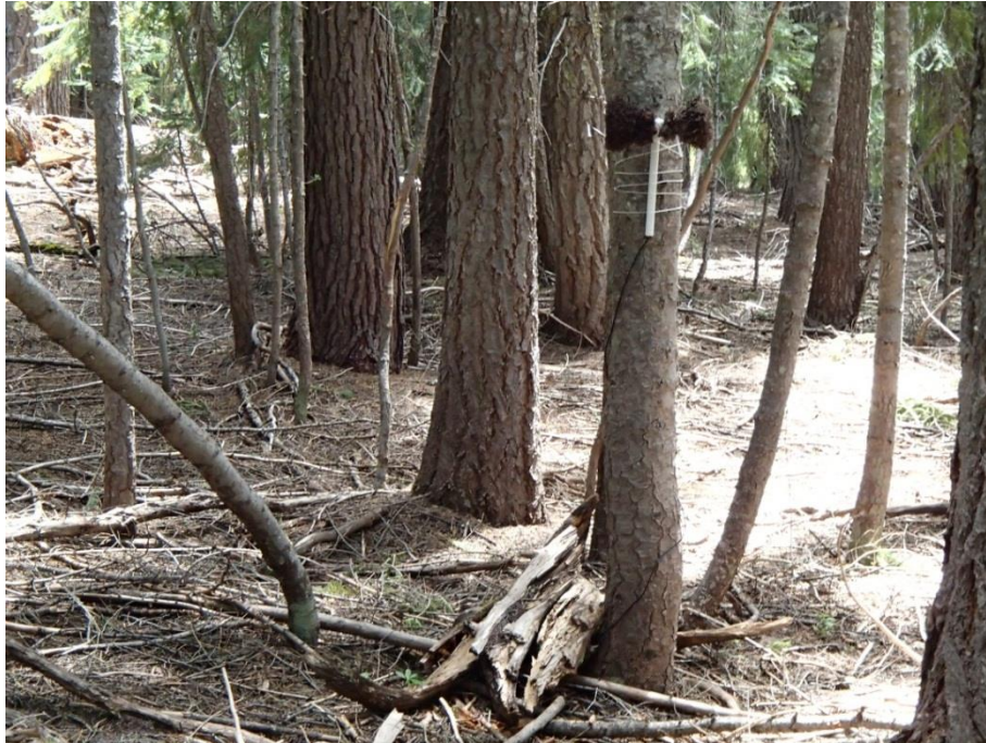
Figure 4. Photograph of a sound station deployed at the Lower Sun Creek Site. The Pelican box is covered with woody debris to prevent being tampered with by wildlife.
