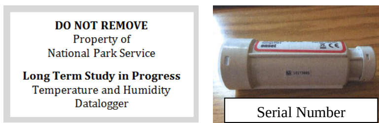
Figure 5-2. Data logger label and location of serial number on the data logger.
