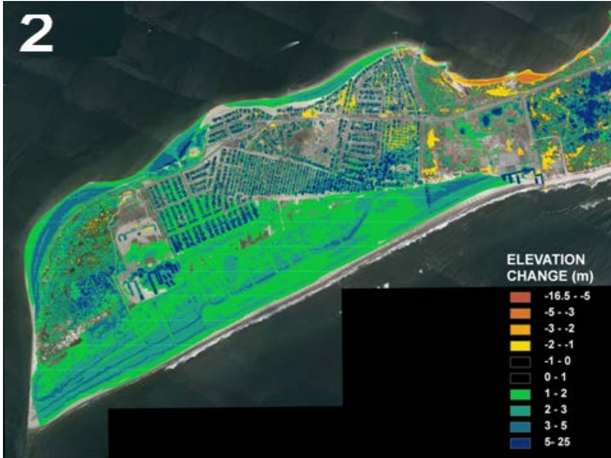
Figure 12. GATE: Example of raster subtraction of historical digital terrain data (1953) from modern LiDAR (2006) data. Cool colors indicate accretion and warm colors indicate erosion.
