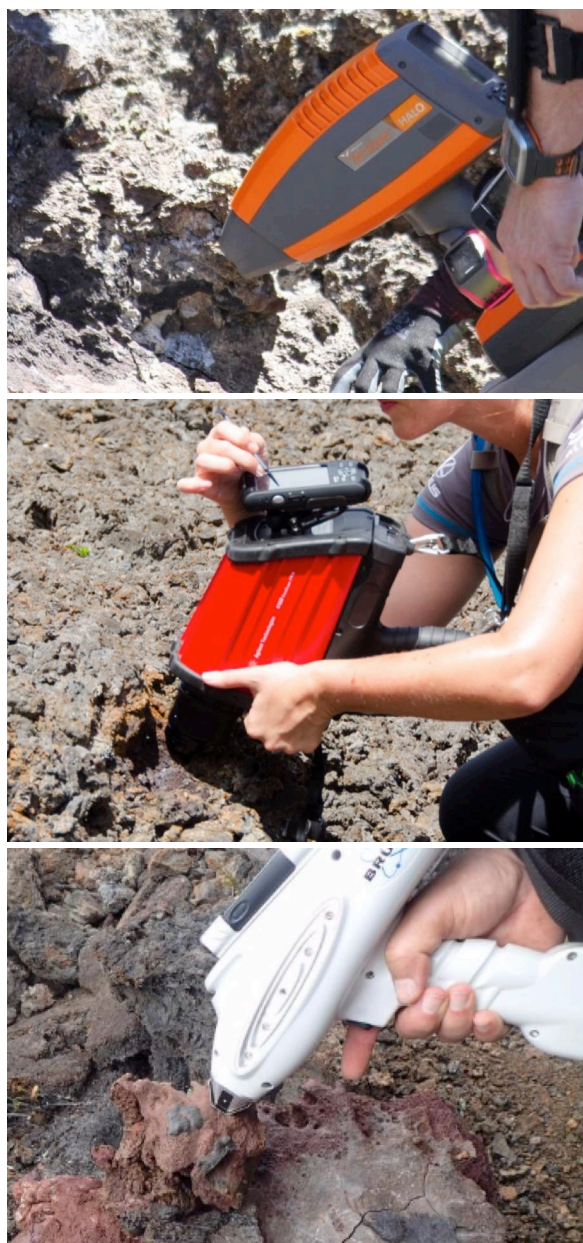
Figure 1: Field instruments used in our study, an ASD TerraSpec® Halo VNIR spectrometer (top), Agilent Exoscan 4100 FTIR spectrometer (middle), and a Bruker Tracer-IV SD XRF spectrometer (bottom).
