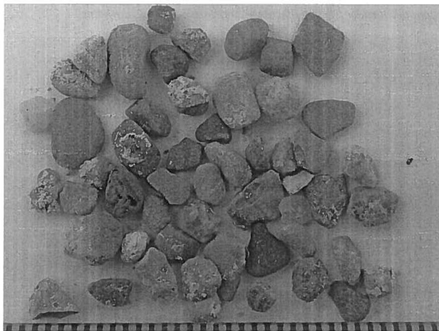
Figure A4: Sample 3736 – Greater than 2.00 mm fraction of extracted and sieved sand, aggregate, and fines; dry condition.
